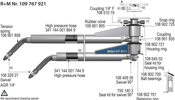
connections once a year for normal wear and tear. No greasing required
